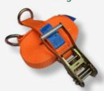
10m Long Strap. Manufactured to BSEN 12195-2:2000. Rated assembly 5000kg. 100% polyester webbing. Orange webbing as standard with single D ring.
