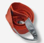
Superior quality 5 Tonne Duplex Webbing Sling Manufactured to BSEN 1492-1:200 from Mudfords With a 7:1 SWL ratio.
