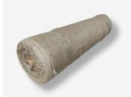
Jute Hessian Scrim for use during the construction of plaster mouldings. Jute Scrim adds strength to the fibrous plaster and prevents cracking. Available in 200m length rolls.
